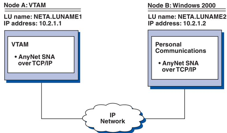
Figure 21. APPC3270 Emulation over a TCP/IP Network
