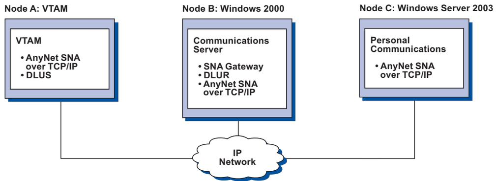
Figure 15. 3270 Emulation via an SNA Gateway over a TCP/IP Network
