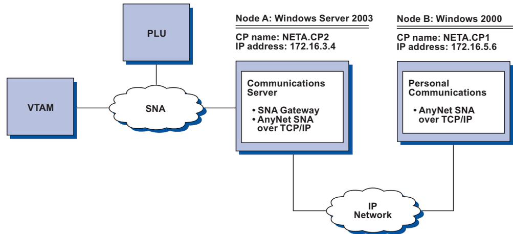
Figure 23. 3270 Emulation over a TCP/IP Network via a SNA Gateway to a VTAM Host on an SNA Network
