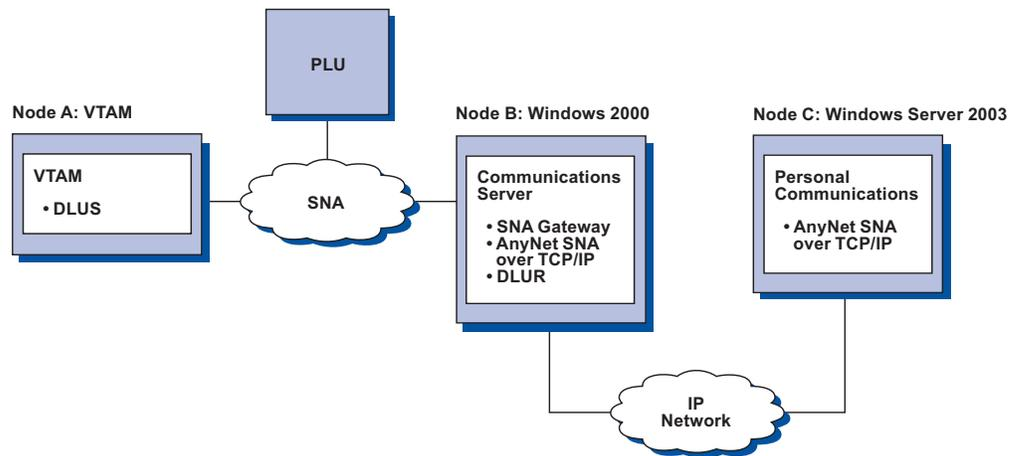
Figure 14. 3270 Emulation over a TCP/IP Network via an SNA Gateway to a VTAM Host on an APPN Network
