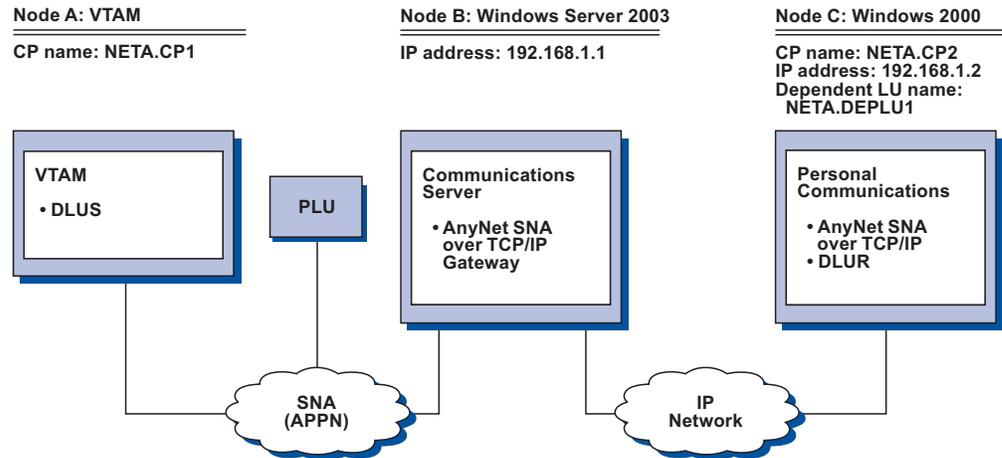
Figure 25. 3270 Emulation over a TCP/IP Network via an AnyNet SNA/IP Gateway to a VTAM Host on an APPN Network
