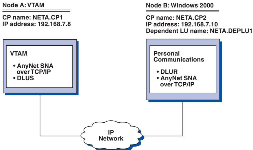
Figure 22. 3270 Emulation via DLUR over a TCP/IP Network
