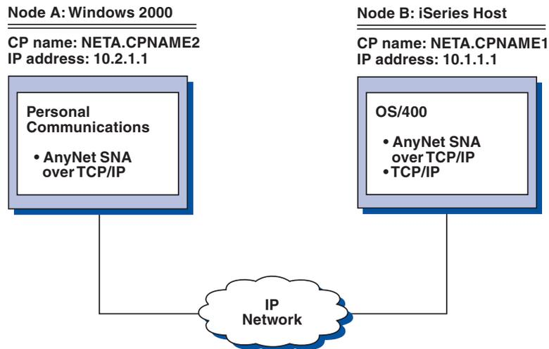
Figure 19. 5250 Emulation Over a TCP/IP Network
