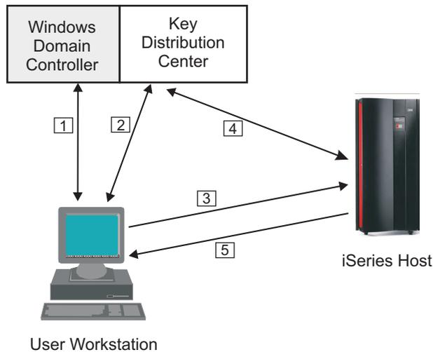
Figure 3. Logging onto a network using Kerberos-based authentication
