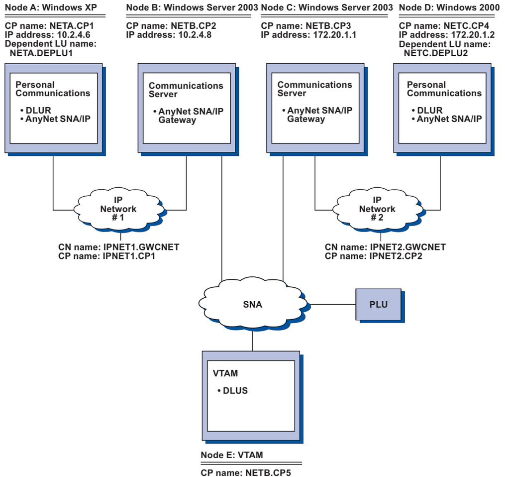
Figure 26. 3270 Emulation on Different IP Networks
