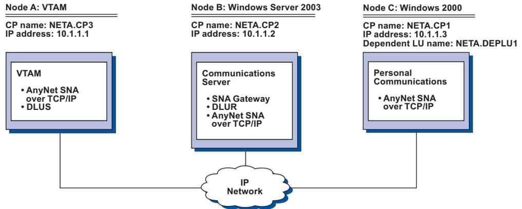
Figure 24. 3270 Emulation via an SNA Gateway over a TCP/IP Network
