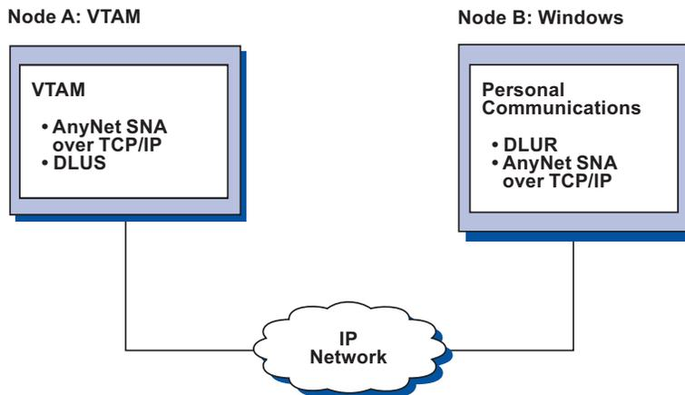
Figure 12. 3270 Emulation via DLUR over a TCP/IP Network
