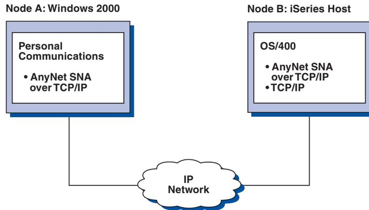
Figure 10. 5250 Emulation over a TCP/IP Network
