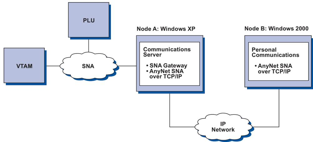
Figure 13. 3270 Emulation over a TCP/IP Network via an SNA Gateway to a VTAM Host on an SNA Network
