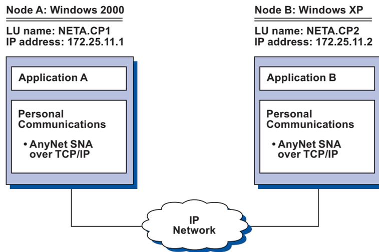
Figure 20. Running APPC or CPI-C Applications over a TCP/IP Network
