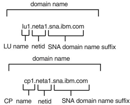
Figure 17. Formats of the Domain Names That SNA over TCP/IP Builds
