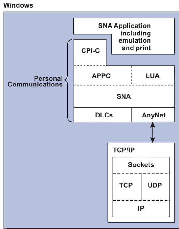
Figure 16. Structure of SNA over TCP/IP for Personal Communications
