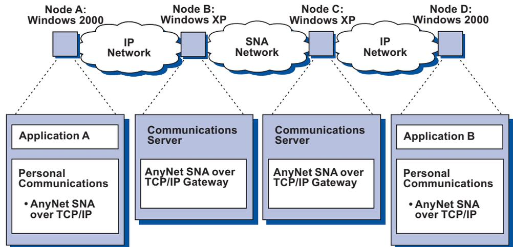
Figure 9. Chaining Multiple Gateways to Connect Multiple IP Networks
